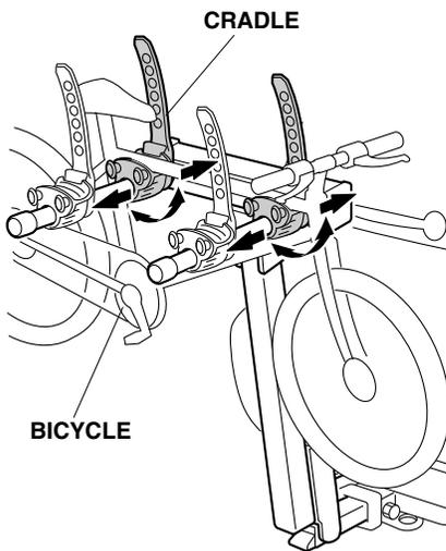
2. Install the two anti-sway cage assemblies to the bicycle arms as shown.
