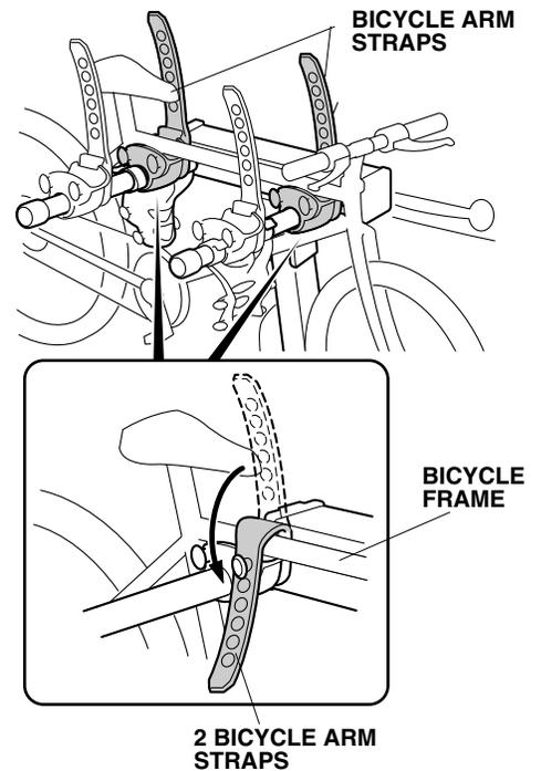
4. Install the two anti-sway straps. Tighten each anti-sway strap securely around the bicycle frame.
